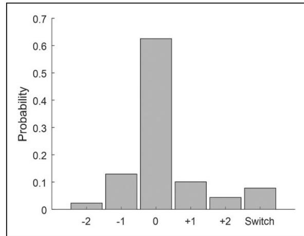
**Figure 7.** Histogram representing the accuracy of the EOG-steering algorithm detailing the distribution of correct (0) and incorrect decisions ( $\pm 1$ ,  $\pm 2$ , switch), including error bars ( $\pm SD$ ).
