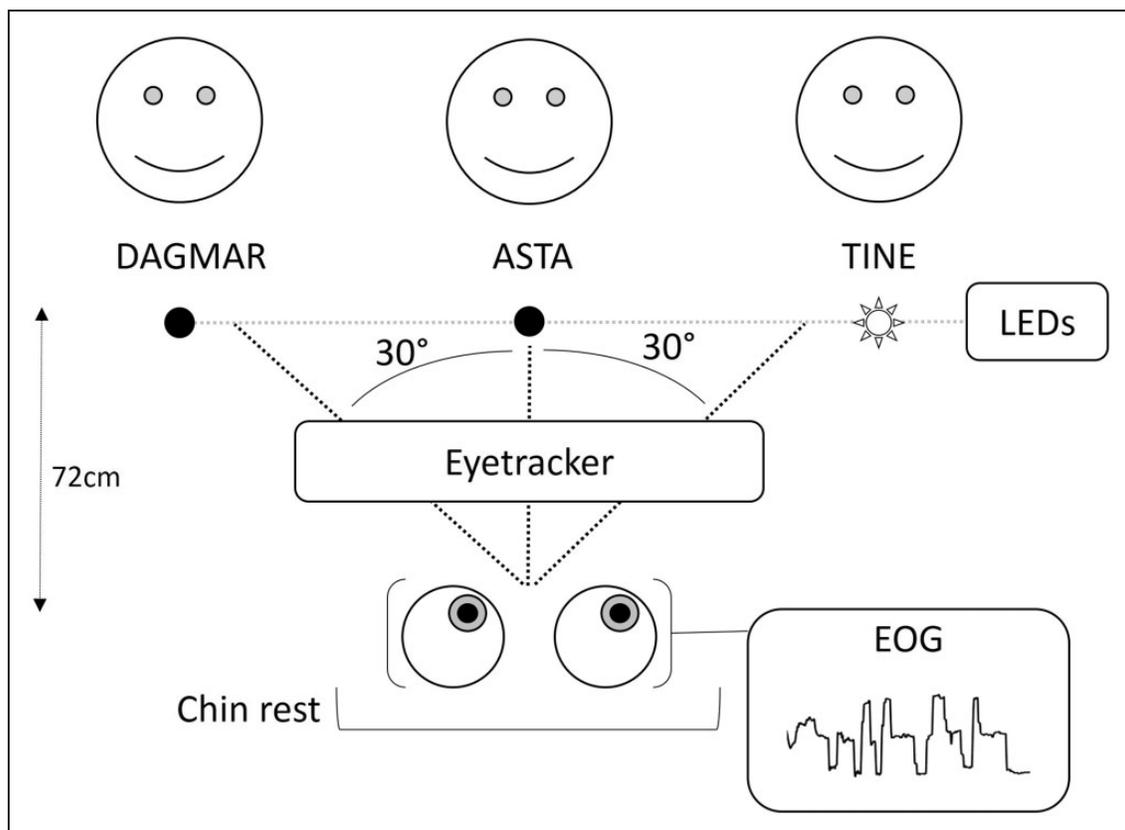
**Figure 2.** Representation of the experimental setup. There were three talkers, one target talker indicated by an active LED (Tine in this example), and two interfering talkers in front of the participant. The head was fixed with a chinrest, and the eye gaze was measured with an eye-tracker and estimated via EOG.
