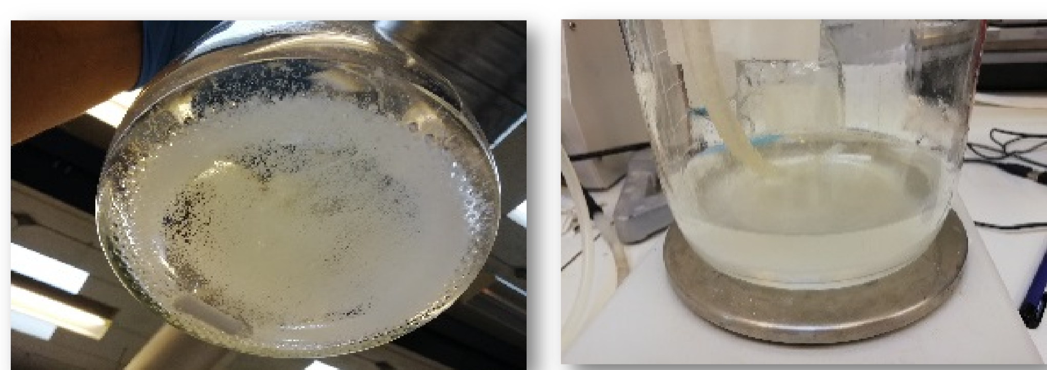
Figure 4. Succinic acid up-concentration and crystallization at pH 3.
