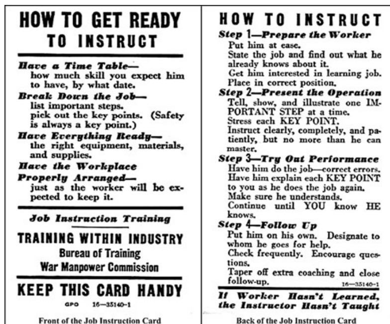
Figure 2: A card for the trainer contains a description of the training method. There are four training steps (prepare, present, perform and follow-up) and is guide that the trainer follows to provide a comprehensive training (Dooley 2001).
