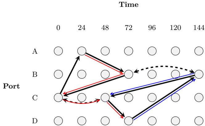
Figure 1: Illustration of a time-space graph  $G$ . Solid arcs represent sailings between ports and dashed arcs represent transshipments. The colored arcs denote examples of cargo paths; the blue path from port D to port C is direct, whereas the red path from port A to port D requires a transshipment at port C. Backward arcs represent sailings or transshipments that end in the following week.
