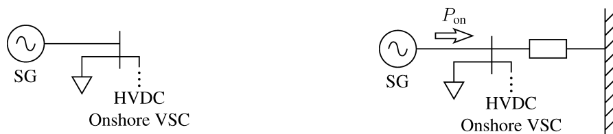
Figure 2-3: Onshore AC network models for onshore FS (left) and POD (right) studies
