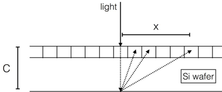
**Figure 3.** The figure shows a schematic representation of our hypothesis for the nature of the observed effect and how it affects the registration of radiation in one pixel. Part of the light incident on the CCD penetrates the pixel layer without giving rise to a signal, and instead reflects off the backside of the CCD eventually resulting in an additional signal being registered at a distance  $x$  from the pixel receiving the incident light.  $C$  is the bulk thickness of the CCD.
