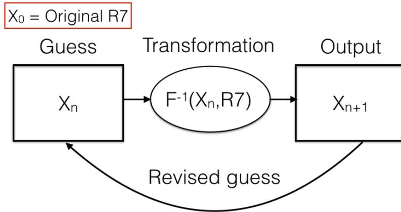
**Figure 5.** This schematic shows how the R7 images are corrected using an iterative process. Each iteration consists of a full circle in the schematic and results in an output which is a fully transformed image one pixel at a time. This output is then used as the new guess in the following iteration. The output will converge, and when a certain pre-defined cut-off value is reached, the iterative process will stop.
