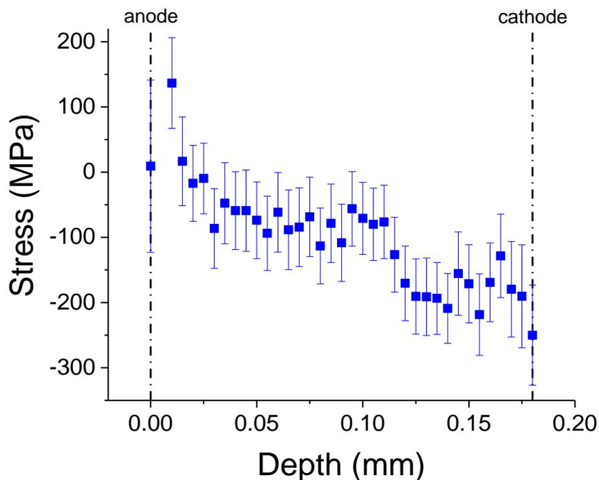
Figure S5. Expected stress across the cell after 24 hours under 2V and 700 °C, assuming that the change in d-spacing is only related to stress.
