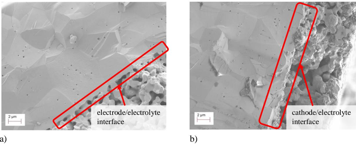
Figure S3. No void formation found in a) sample subjected to 850 °C for 72 hours without applied voltage and b) cathode/electrolyte interface of the sample subjected to 900 °C for 72 hours at 2V. All samples correspond to the 6μm-ScYSZ case and the cathode is made of LSM/YSZ. The interfaces in both cases are marked in the red rectangle.
