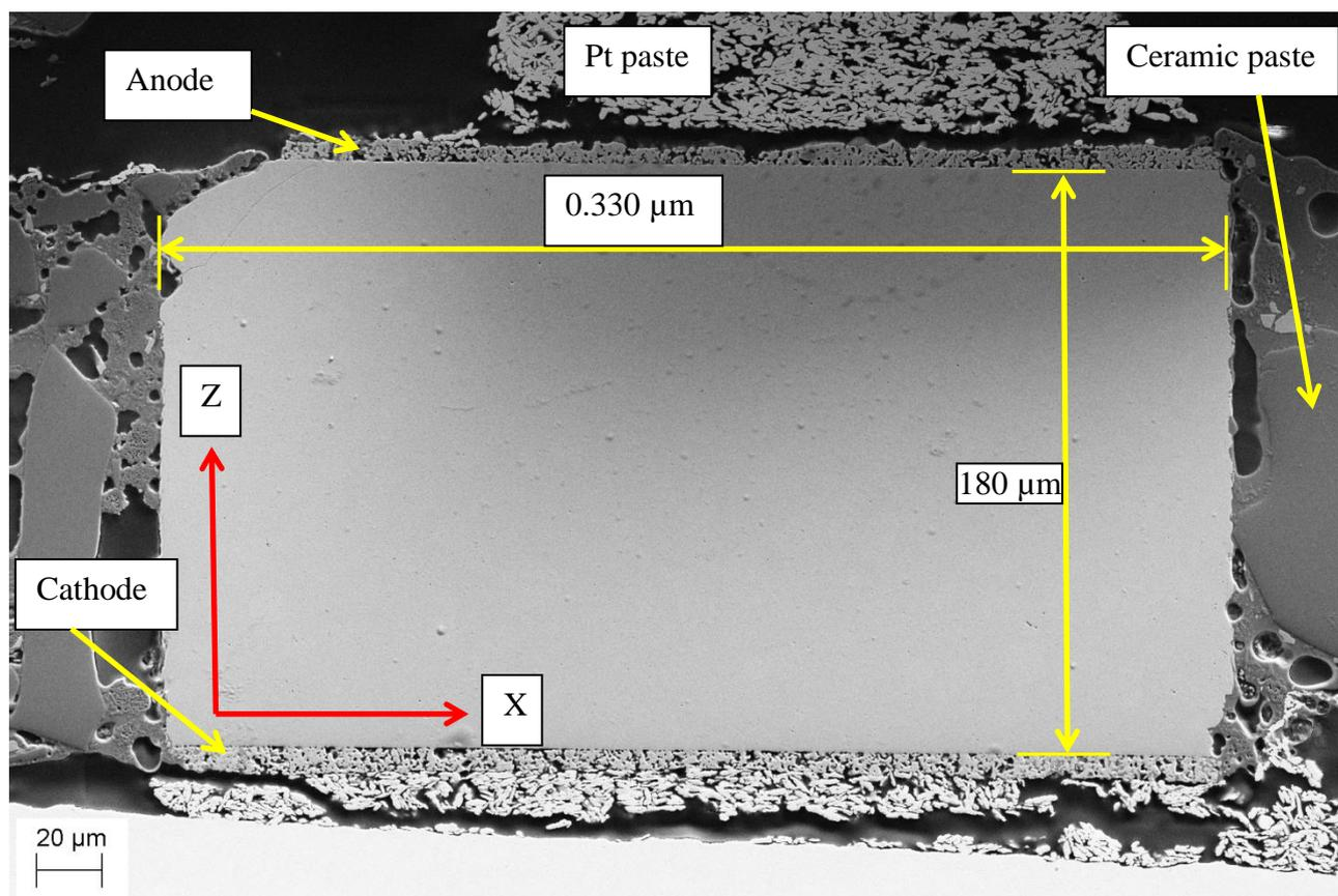
Figure S1. SEM image from a polished cross section of the cell. Directions “X” and “Z” as in beamline setup are denoted by red arrows. Vertical and horizontal dimensions are specified by text boxes next to the corresponding yellow lines delimiting the electrolyte. Yellow arrows attached to text boxes indicate the materials of the cell and cell support.
