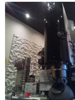
Figure 2. Our environmental transmission electron microscope (ETEM) equipped with built-in gas injection system and gas cell, allowing operation at high pressures.
