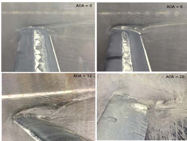
Figure 6: Visualisation of flow structures at the wind tunnel walls for Re = 200,000 at different angles of attack.
