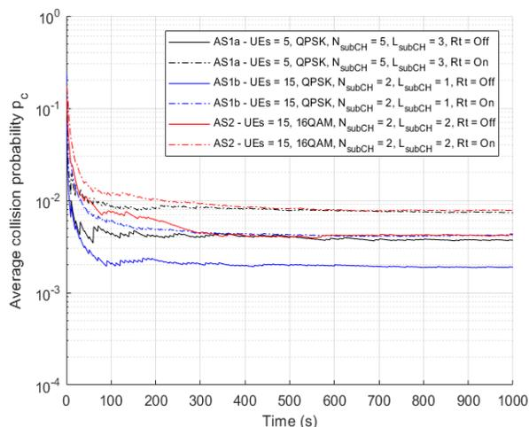
Figure 9. Average collision probability for different application scenarios (ASs)
