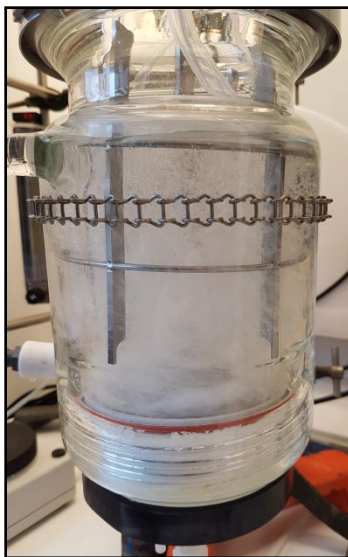
Figure 5. Gas dispersion in the MSMPR crystallizer. The picture was taken on an undersaturated API solution at 10 °C. Agitation speed: 800 rpm. Flow rate (bottom injection): 2.5 L/min.
