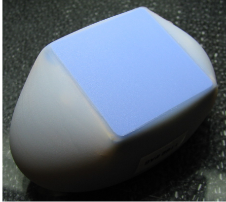
Figure 5.16: The finished nose piece after lensing. The RTV silicone used in this case is blue.
