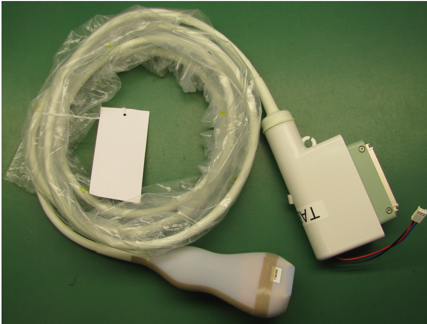
Figure 5.21: The final assembled RCA CMUT probe ready to be connected to the scanner.
