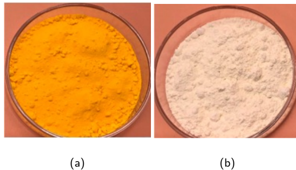
Figure 7.12: \text{Bi}_2\text{O}_3 powder in (a): \beta -phase and (b): \alpha -phase. The powder was bought in \beta -phase, but could be changed to \alpha -phase by a heat treatment.
