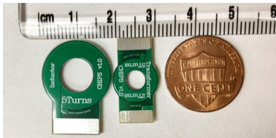
Fig. 10. A photo of inductor and transformer PCB winding prototypes.
