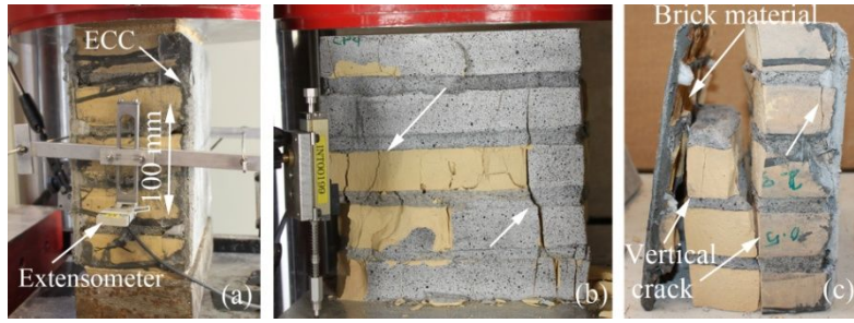
Figure 2.5. (a) Test setup, failure mode of the brick prisms: (b) without strengthening layer, (c) with two layers of ECC
