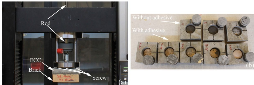
Figure 2.4. (a) Test setup (b) the test specimens after failure in tension
