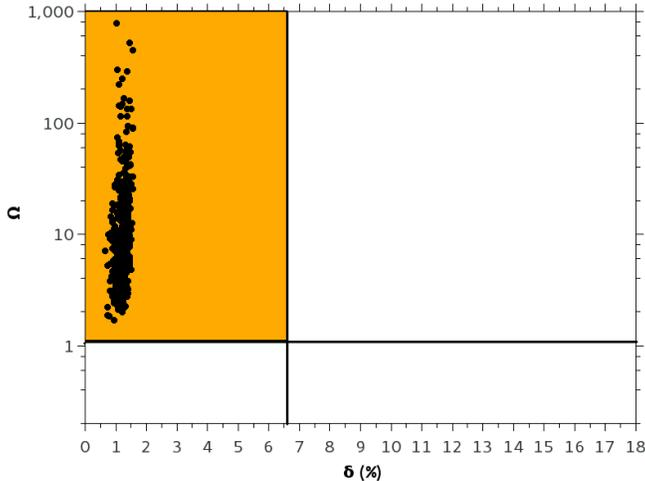
**Figure 1:** A graph of omega values vs delta values for each 8-atom bulk HEA unit cell. The distribution of data shown is well within the theoretical solid solution requirements of  $\delta \leq 6.6\%$  and  $\Omega \geq 1.1$  [23]
