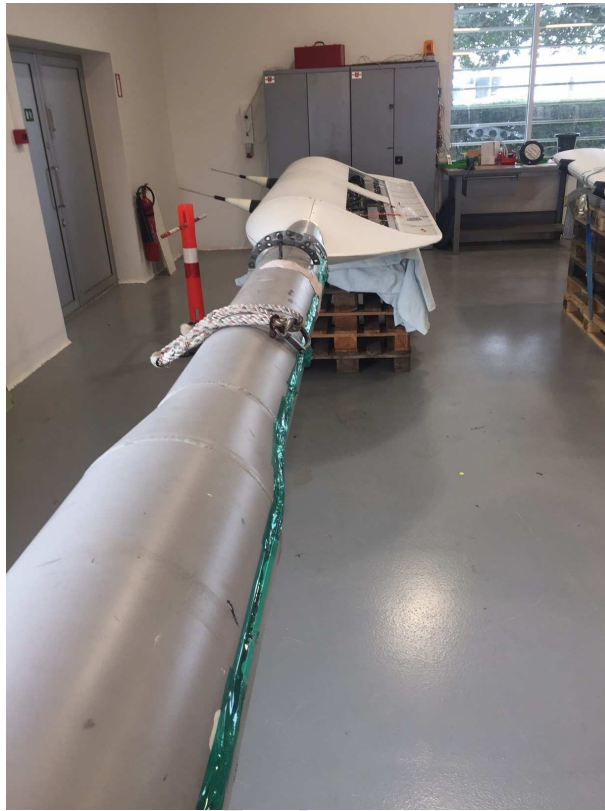
Figure 6: The turbine blade section fitted with morphing flaps and mounted on the boom before installation.
