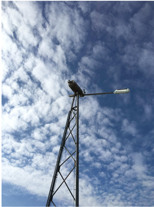
Figure 7: The blade section and the boom installed on the outdoor rotating rig.
