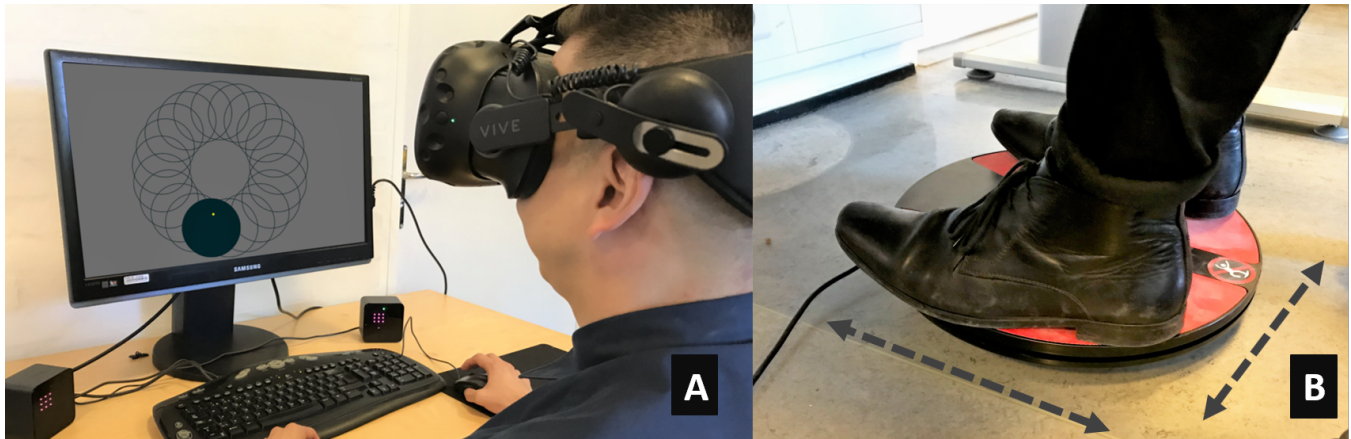
Figure 1: A. Participant with an HTC VIVE headset (HMD) equipped with the Pupil Lab's binocular gaze tracking unit (used for gaze input). The Fitts' multi-directional selection task that the participant is performing inside the headset is also shown on the monitor. The headset also tracks orientation of the head (used for head input). B. Feet on a 3DRudder foot mouse with 360° of movement control (used for foot input). Tilting the 3DRudder moves the cursor in that direction.
