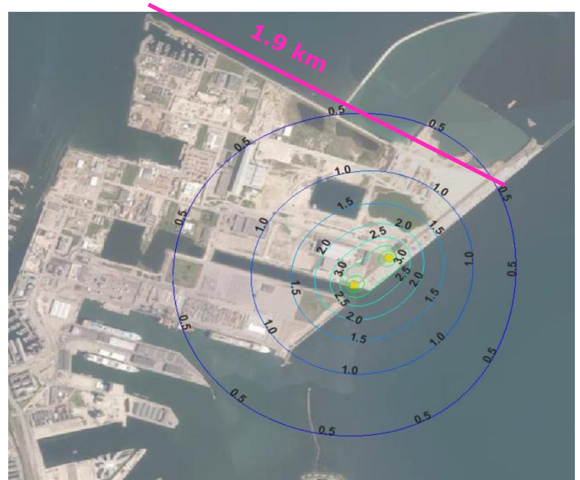
Temporary reduction of groundwater level for 50 m 3 /h
