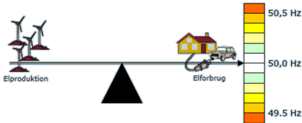
Figure 1: Illustration of the TSO challenge of balancing consumption with variable production.
