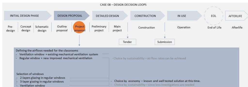
Figure 4 – Case 08 design decision loops, the dark blue arrow illustrates the design phase of which the project is at the time for case study at JJW, the dark blue box contains the design decision loops and the orange dot indicate the phase for interaction with the PhD researcher and the technical inputs.
