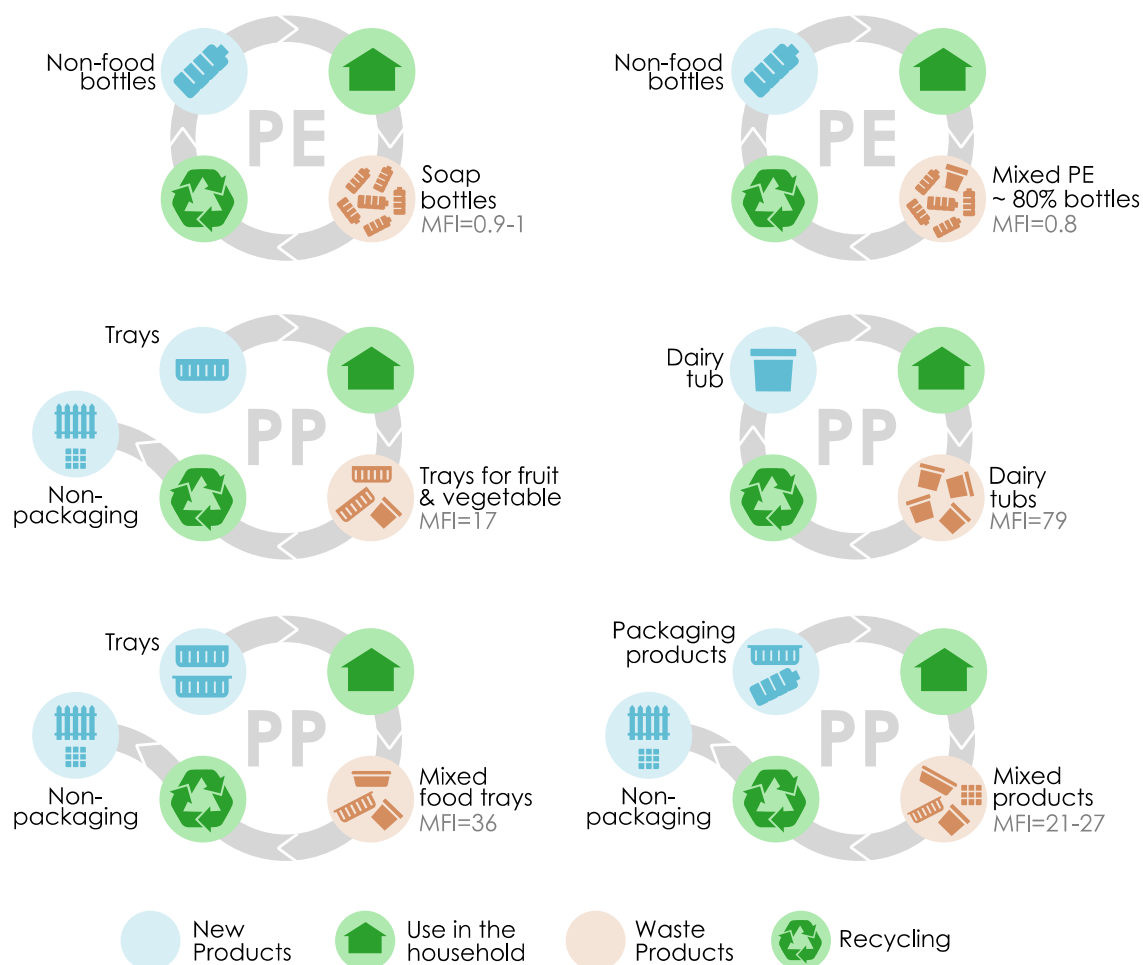
Figure 11 Illustration of potential recycling pathways for different waste products, based on the melt flow index (MFI) of the recycled plastic they can produce, determining the processing method and suitable products, as presented in Table 4. All results are presented in Eriksen et al. IV .
