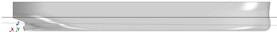
Figure 1: Hull geometry. The upper horizontal line is the water line of the design condition, and the lower horizontal line is the water line of the sea trial condition. Seen from starboard side.
