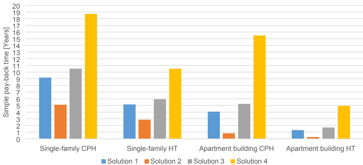
Fig. 4. Simple payback time for customers' investments in improved heating system control in Copenhagen (CPH) and Høje Taastrup (HT).
