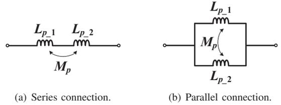
Fig. 2. Series and parallel connection of partial inductance.
