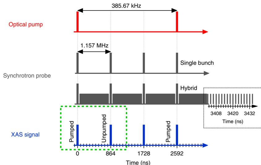
**Fig. 1** Scheme of the pump-probe set-up. Temporal distribution of laser (red) and synchrotron (grey) pulses and of the detected X-ray absorption (XAS) signal (blue). The green dashed box indicates the standard acquisition frame
