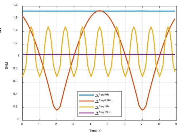
Figure 4 - Time resolved SVM for two superposition square shaped waveforms at 500 Hz and 500+ $\Delta$ freq Hz for four different  $\Delta$ freq.
