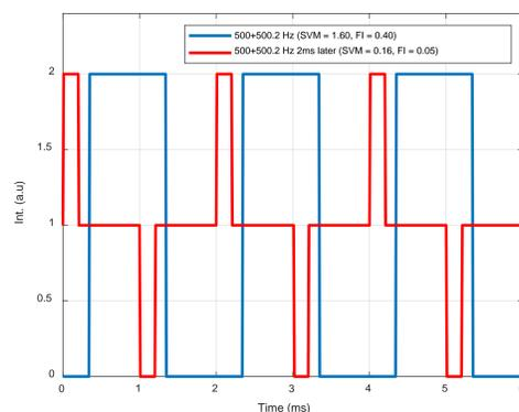
Figure 3 - Superposition of two square shaped waveforms of 500 Hz and 500.2 Hz, at two different positions in time, generating different TLA values (shown in the legend).
