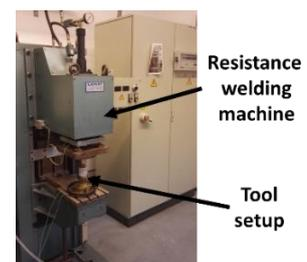
Figure 2: Electrical resistance welding setup.
