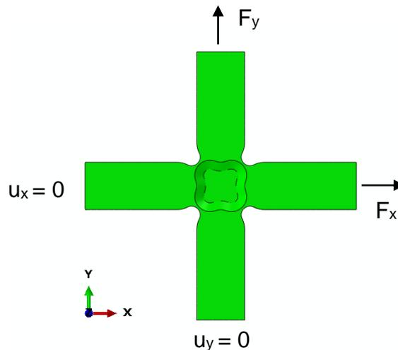
**Figure 4.** Boundary conditions and applied forces to the cruciform specimen.
