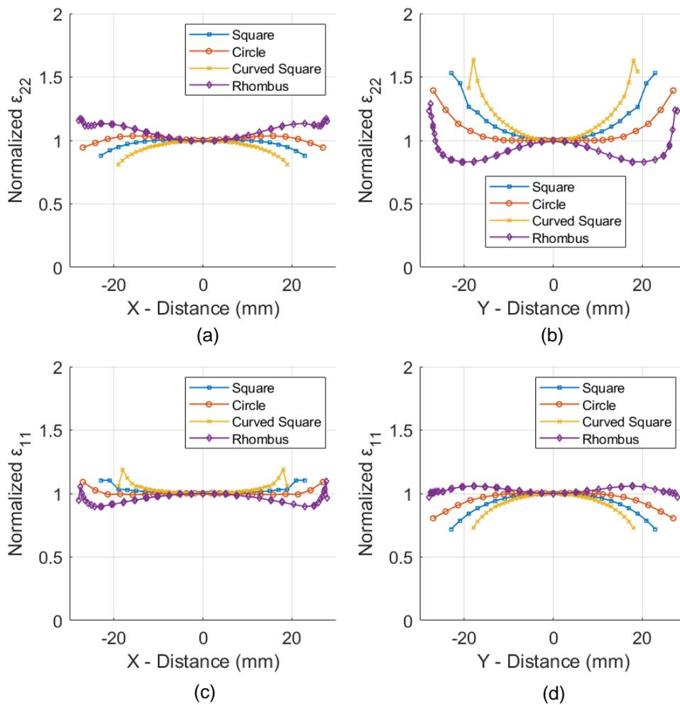
**Figure 6.** Plots for induced biaxial strain state of  $\varepsilon_{xx} = 0.005$  and  $\varepsilon_{yy} = 0.0025$  (a) Normalized  $\varepsilon_{22}$  strains along the X distance in the biaxial zone (b) Normalized  $\varepsilon_{22}$  strains along the Y distance in the biaxial zone (c) Normalized  $\varepsilon_{11}$  strains along the X distance in the biaxial zone and (d) Normalized  $\varepsilon_{11}$  strains along the Y distance in the biaxial zone.
