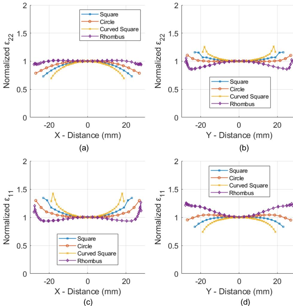
**Figure 7.** Plots for induced biaxial strain state of  $\epsilon_{xx} = 0.0025$  and  $\epsilon_{yy} = 0.005$  (a) Normalized  $\epsilon_{22}$  strains along the X distance in the biaxial zone (b) Normalized  $\epsilon_{22}$  strains along the Y distance in the biaxial zone (c) Normalized  $\epsilon_{11}$  strains along the X distance in the biaxial zone and (d) Normalized  $\epsilon_{11}$  strains along the Y distance in the biaxial zone.
