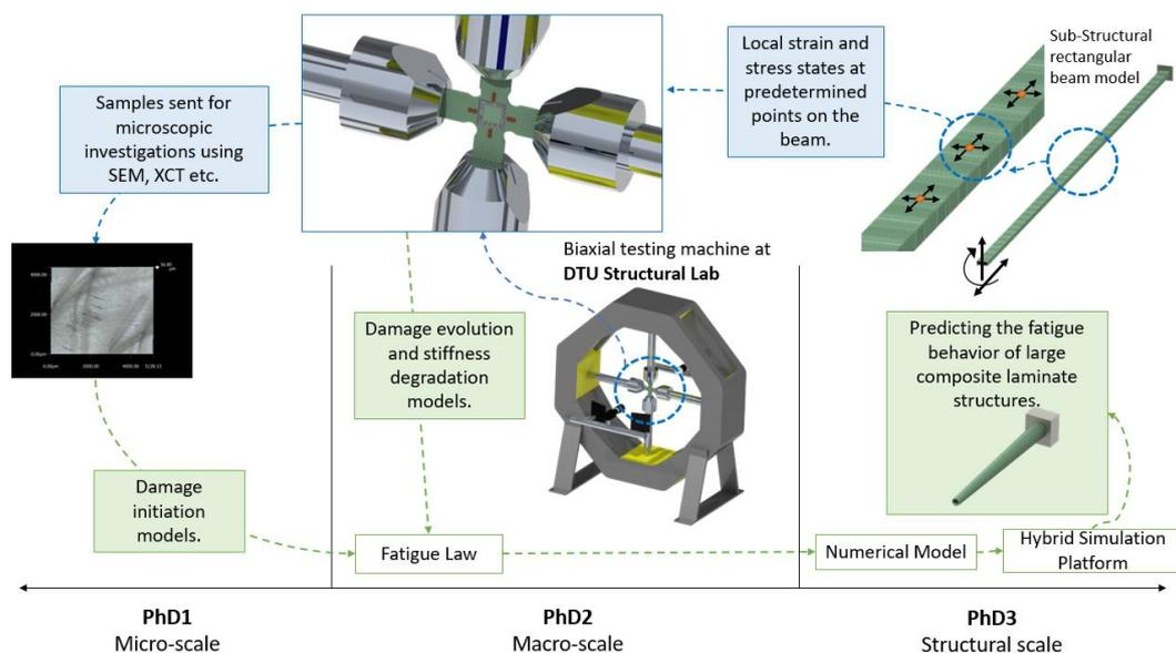
Figure 1. Multi-scale testing and modelling approach.
