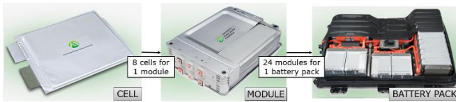
Figure 2. From the single cell to the battery pack. Adapted from Nissan.
