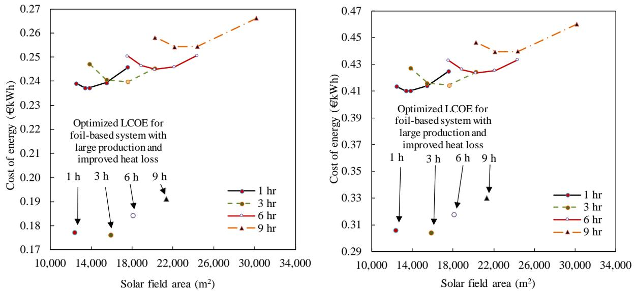
Figure 3b. Variations in LCOE with foil-based solar field area. Discount rates: 3 % (left figure) and 10 % (right figure).
