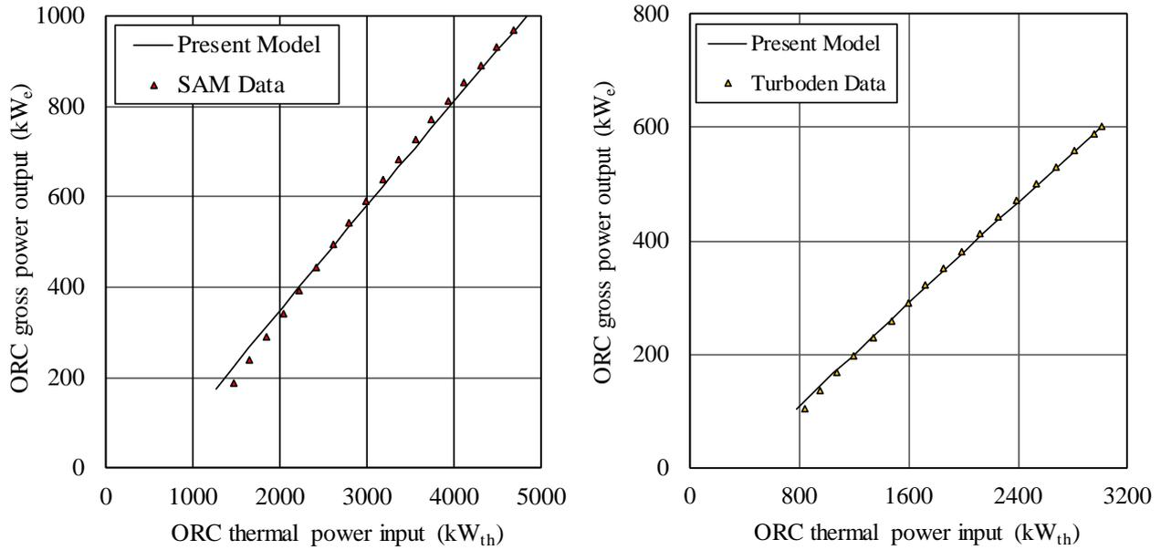
Figure 2. Comparisons between the ORC power system performance using (i) System advisor model (SAM) for the 1 MW APS Saguaro plant and the present model (left figure) and (ii) Turboden data for a 600 kW plant and the present model (right figure).
