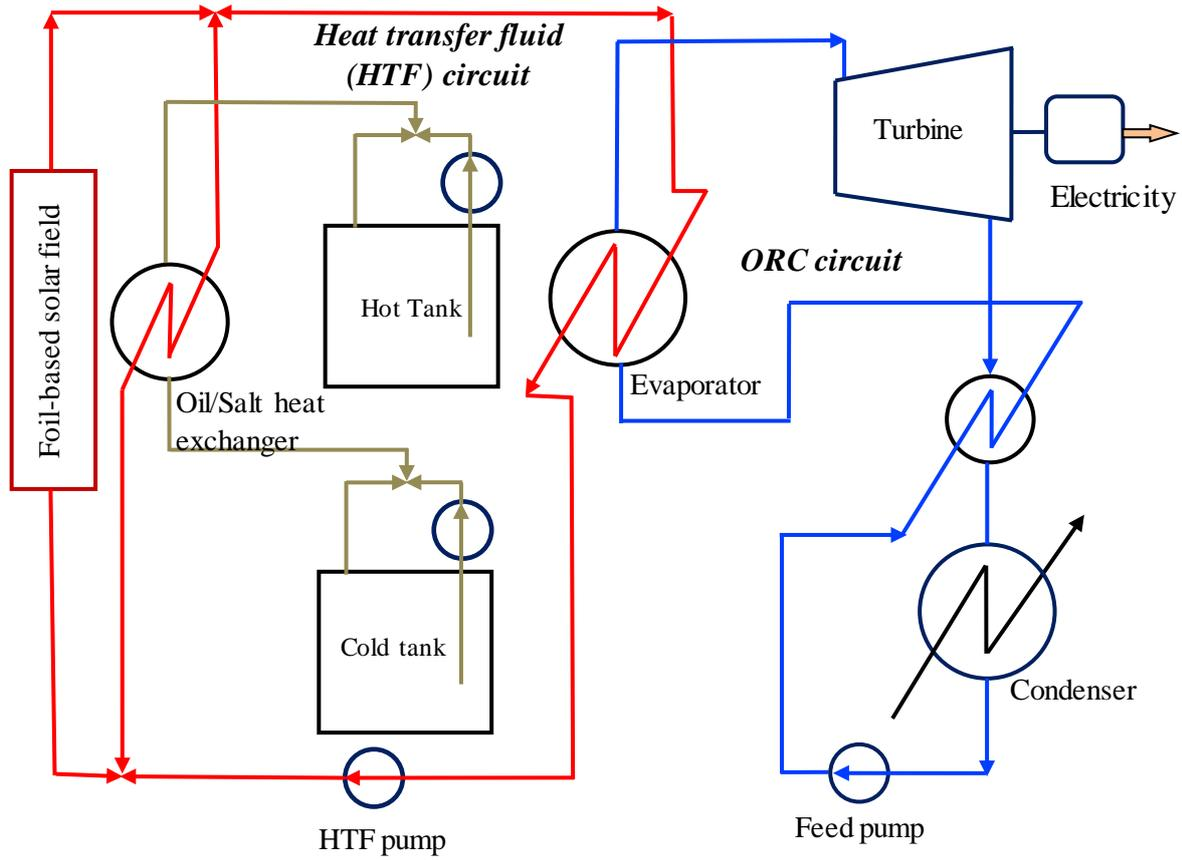
Figure 1a. Foil-based concentrating solar collector powered organic Rankine cycle system.
