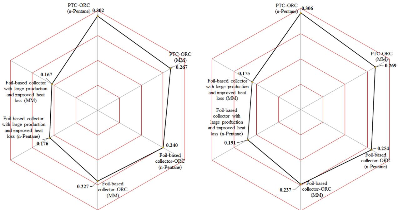
Figure 4. Comparisons of LCOE with discount rate 3 %. Storage capacity: 3 h (left figure) and 9 h (right figure).
