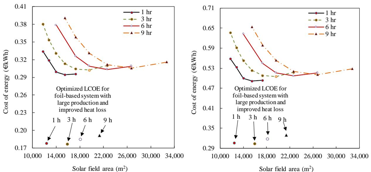
Figure 3a. Variations in LCOE with PTC area. Discount rates: 3% (left figure) and 10% (right figure).
