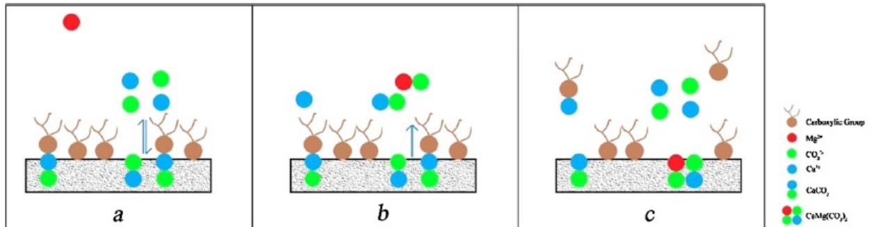
**Figure 1** Proposed mechanism of wettability alteration of a carbonate rock surface by  $Mg^{2+}$  (from Rashid et al. (Rashid et al., 2015)).
