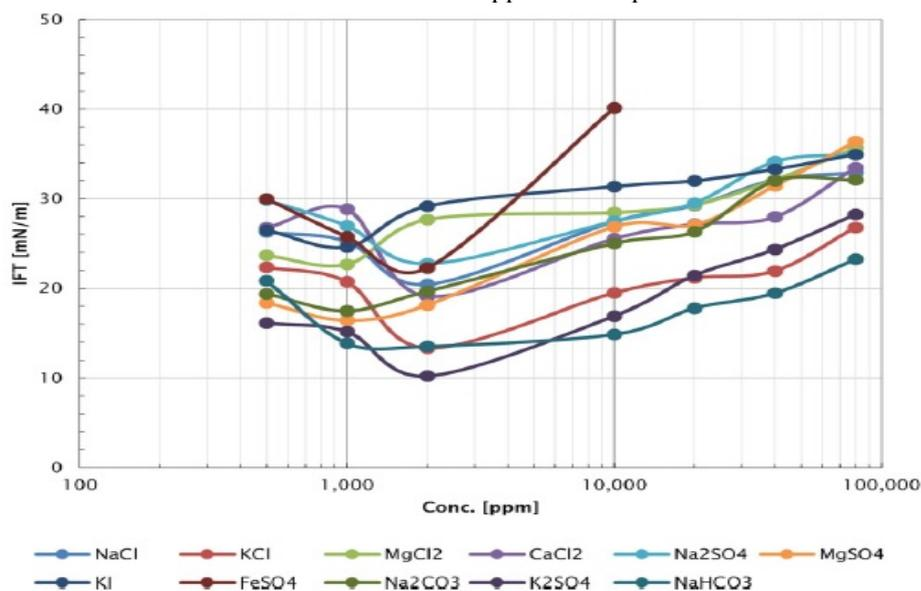
**Figure 2** The interfacial tension (IFT) between oil and salt solutions against concentration at reservoir temperature and atmosphere pressure (from (Khaksar Manshad et al., 2016)).
