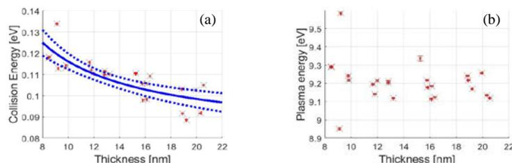
**Fig. 1** The fitted values of the collision (a) and plasma (b) energy from the measured ellipsometer data. The full line is the best fit with the  $1/t$  dependence. Dotted lines show the 95% confidence interval. The computed error bars (red lines) are too small to be visible. The fitting was made between 675 to 1750nm, to minimise the influence of the Lorentz terms.
