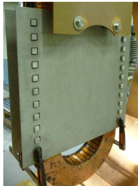
Fig. 7. Full coil with mechanical support during mounting in cryostat.
