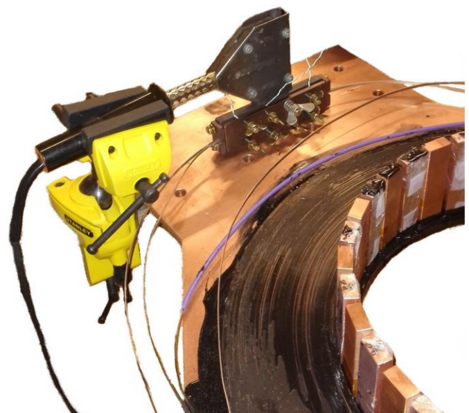
Fig. 4. Stacking of double pancake coils No.1 and 2, and using the spring soldering iron to join the wire ends of the two double pancakes.
