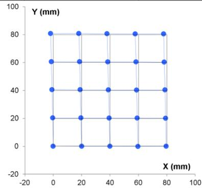
Figure 3. Schematic magnified error (100x) of the average position for each of the 25 measured holes of the CLIP manufactured specimens.
