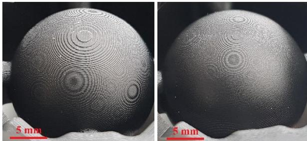
Figure 2. Manufactured  $\varnothing 22\text{mm}$  spheres: sphere #1 with slicing layer height  $h_1$  to the left and sphere #2 with  $h_2$  to the right.
