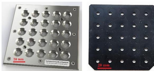
**Figure 1.** Picture showing the Optomechanical hole plate and the CLIP fabricated replicate used for the investigation. The large chamfered corners are facing the CLIP machine operator during fabrication.
