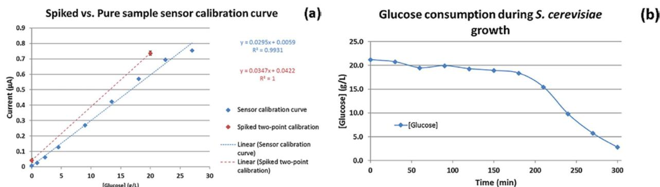
**Figure 1.** Graphite sensor performance with fermentation samples: (a) pure sample calibration curve (dotted line) vs. glucose spiked YPD media two-point calibration (dashed line) and (b) on-line quantification of glucose consumption by *S. cerevisiae* in a micro-bioreactor determined by a glucose biosensor (N = 3). Adopted from Fernandez et al.<sup>4</sup>
