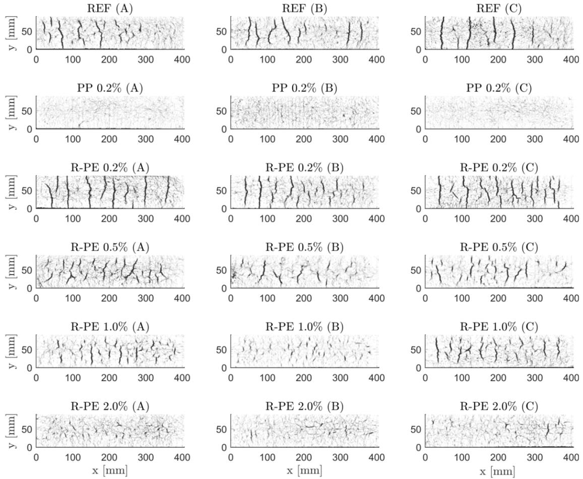
Figure 4: Principal strain for specimens at  $t = 25$  h. White colour represents uncracked area with strain  $\epsilon_{x,y} = 0\%$ ; Black colour represents surface cracks with strain  $\epsilon_{x,y} = 5\%$ .
