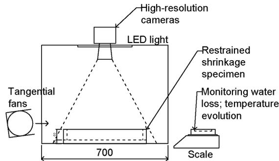
Figure 2: Plastic shrinkage test setup using DIC
