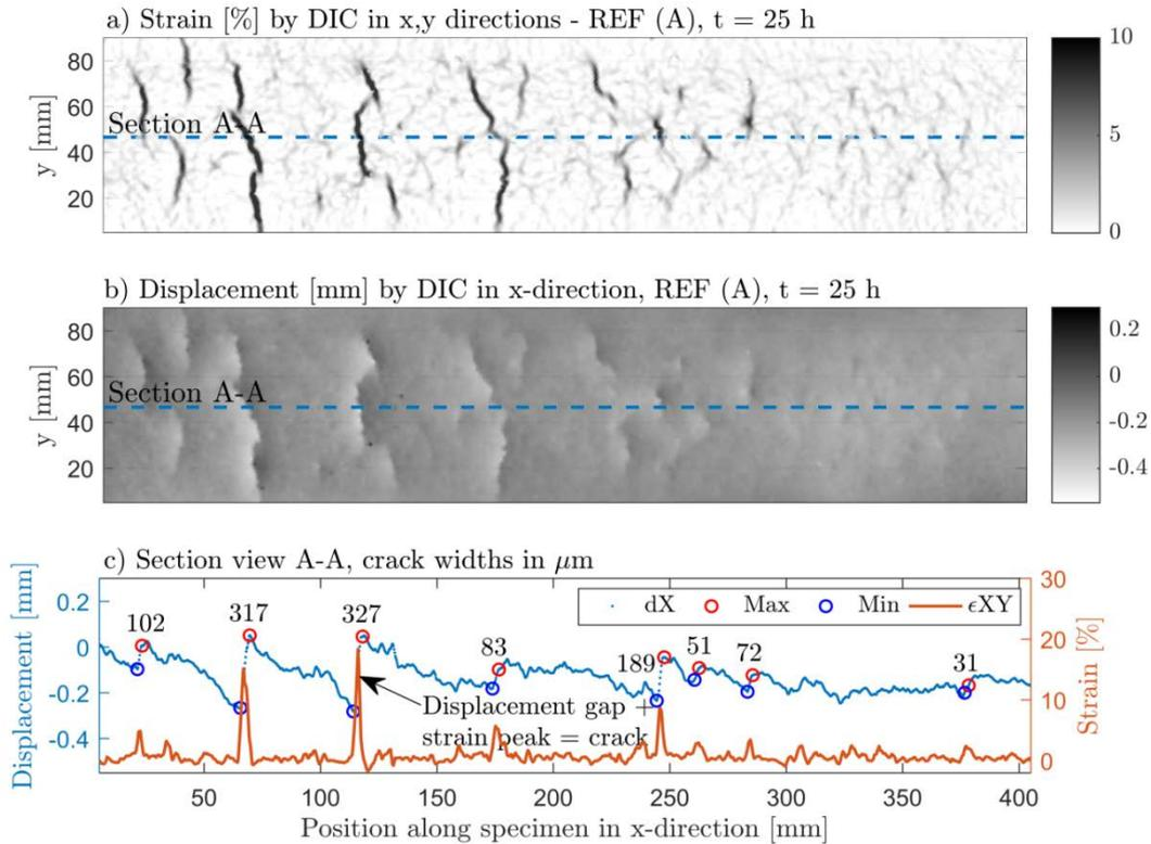
Figure 3: REF (A) specimen at  $t = 25$  h. a) Principal surface strain in the (x,y)-direction by DIC; b) Surface displacement in the x-direction by DIC; c) Section A-A going through specimen showing surface displacement in x-direction and principal strain
