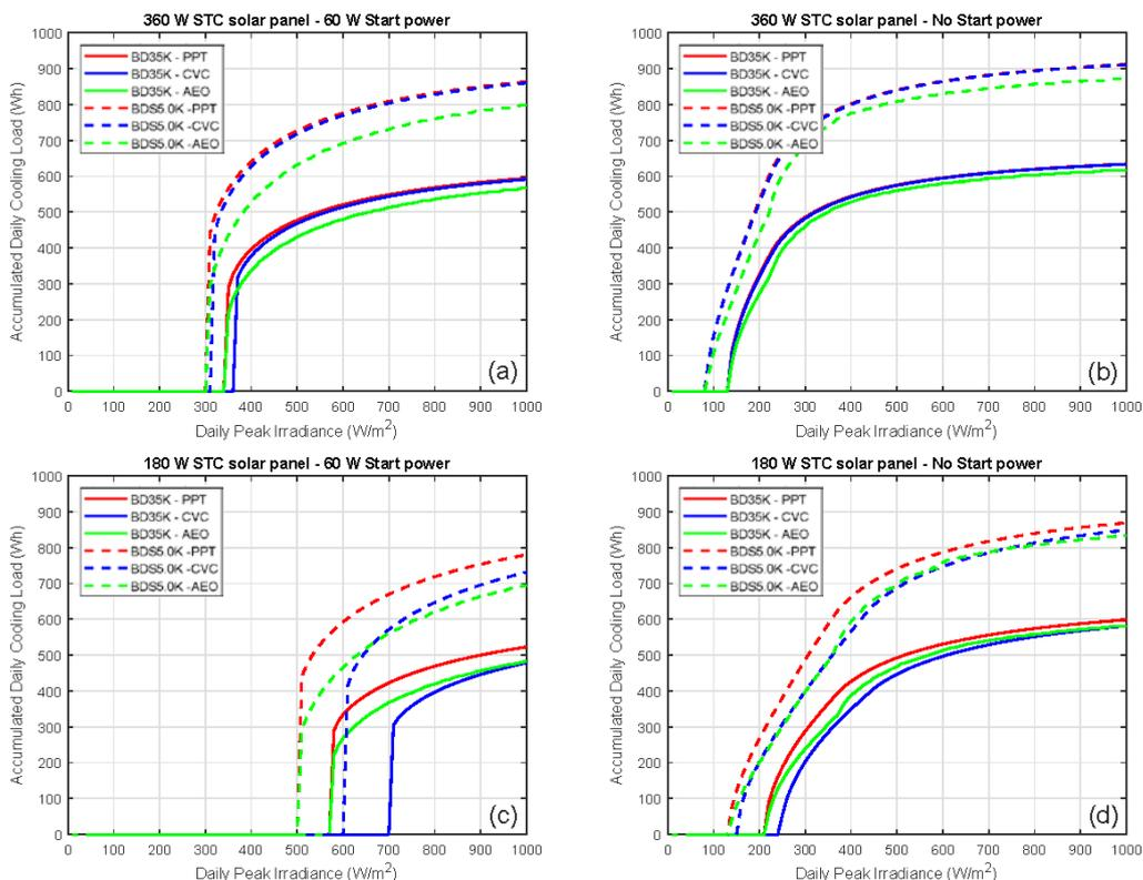
**Figure 6: Daily accumulated cooling for the BD35K and BDS5.0K compressors under the PPT, CVC and AEO control strategies using both the 180 W and 360 W PV panels and with and without compressor start power delivered from the PV panel**
