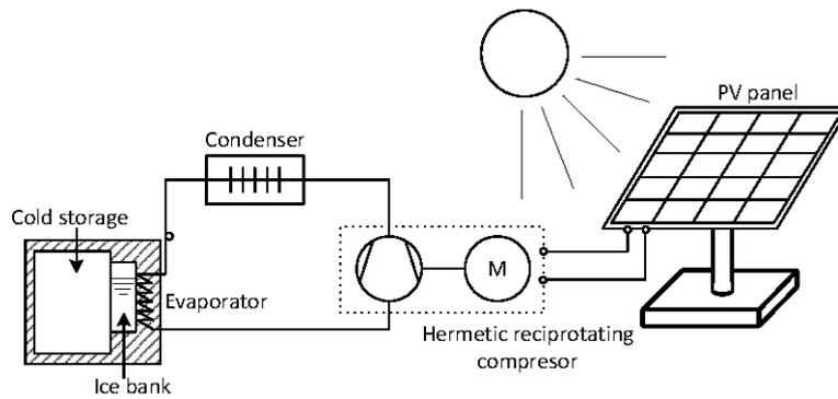
**Figure 1: Principle sketch of the direct drive solar refrigeration system with ice bank storage**
