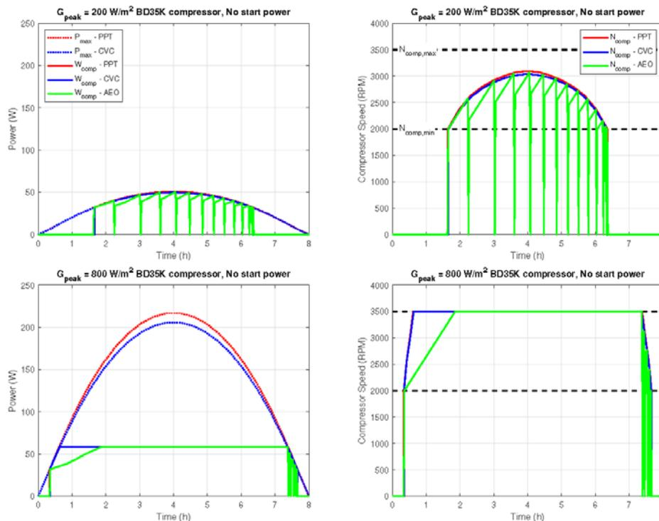
**Figure 4: Compressor power and compressor speed for the PPT, CVC and AEO control strategies under two different irradiance profiles with 200 Wm<sup>-2</sup> and 800 Wm<sup>-2</sup> peak irradiance, respectively. Results are shown for the BD35K compressor without start power**
