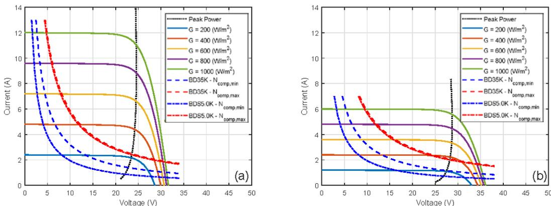
**Figure 3: Current - voltage curves for the 360 W (a) and 180 W (b) PV panels, with the current - voltage curve for the two investigated compressors at their minimum and maximum compressor speeds**
