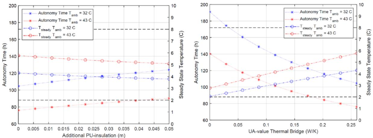
**Figure 4: Autonomy time and steady state temperature as a function of additional PU-insulation in the cabinet walls (left) compared to the baseline model and as a function of the UA-value of the thermal bridges (right)**
