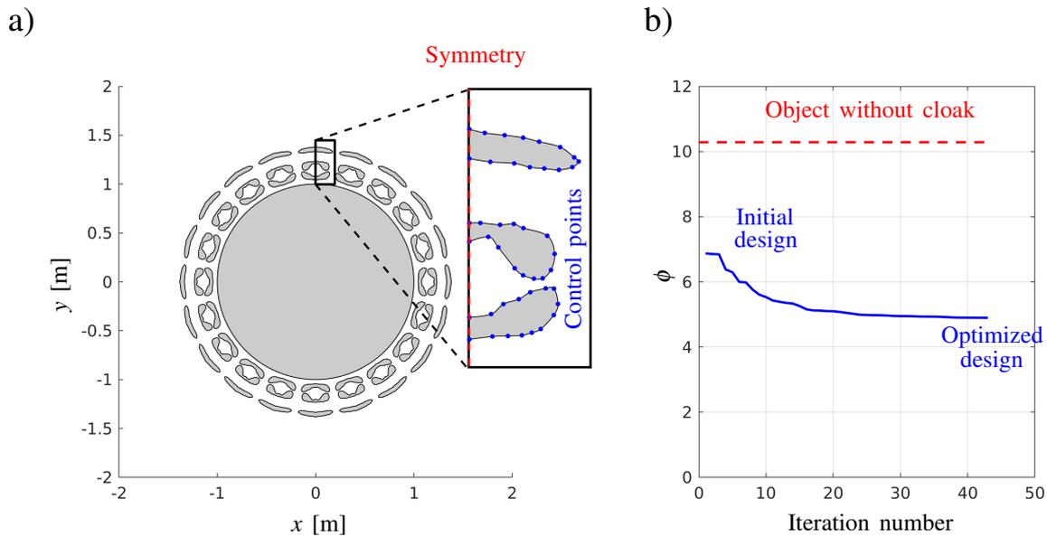
Figure 2. a) Shape-optimized design of the multi-directional cloak, including a magnified area presenting the location of the control points. b) evolution of the objective function  $\phi$  during optimization (continuous blue line). Additionally, the plot includes the value of the objective function when only the cylindrical object is considered (dashed red line).
