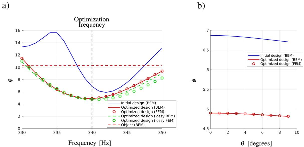
Figure 3. a) Frequency dependence of the objective function for both the initial (blue) and the optimized (red) design. The figure also includes simulations including viscous and thermal losses (green). b) Dependence of the incident angle of the impinging plane wave for the initial (blue) and the optimized (red) design. circular symbols represent equivalent FEM simulations for comparison.
