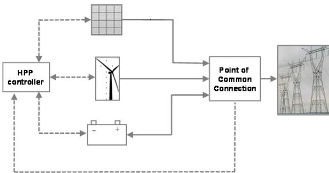
Figure 1: HPP –utility scale co-located grid connected
