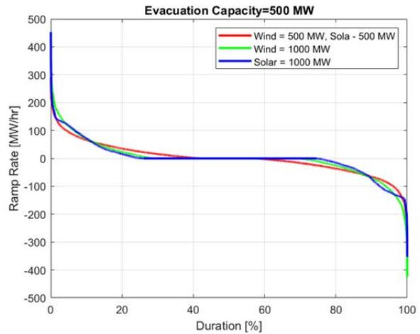
Figure 6 Ramp rate of HPP with total installed capacity = 1000 MW and evacuation capacity = 500 MW
