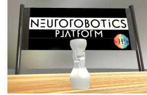
Fig. 3. Experimental set up. One module of the Fable robot arm is fixed to a table in order to avoid undesired dynamics.
