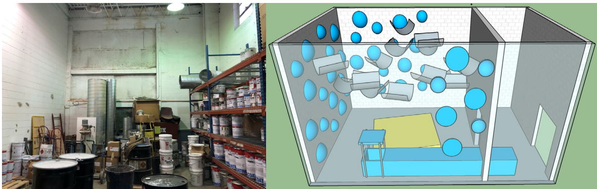
Figure 1(left) Existing space; (right) Rendered rev room rotated counterclockwise 90 degrees with the front wall in Fig. 1 (left) on the left
