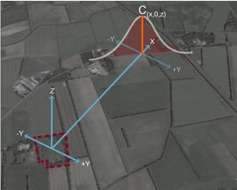
4 Fig. 1. Dispersion model applied to the measured downwind methane plume from a landfill. The height of the red curve 5 is proportional to measured methane concentrations above background level during a traverse of the downwind plume.
