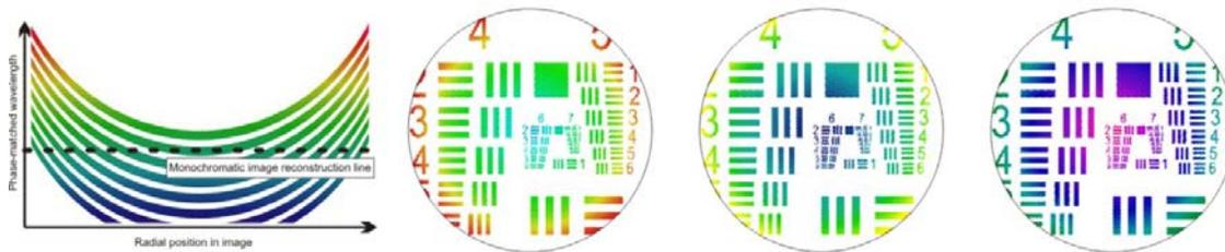
Fig. 2. Scanning of the phase match condition of the frequency conversion process enables acquisition of the spectral response in each pixel element of the image plane. Post-processing is needed to extract monochromatic images [10].
