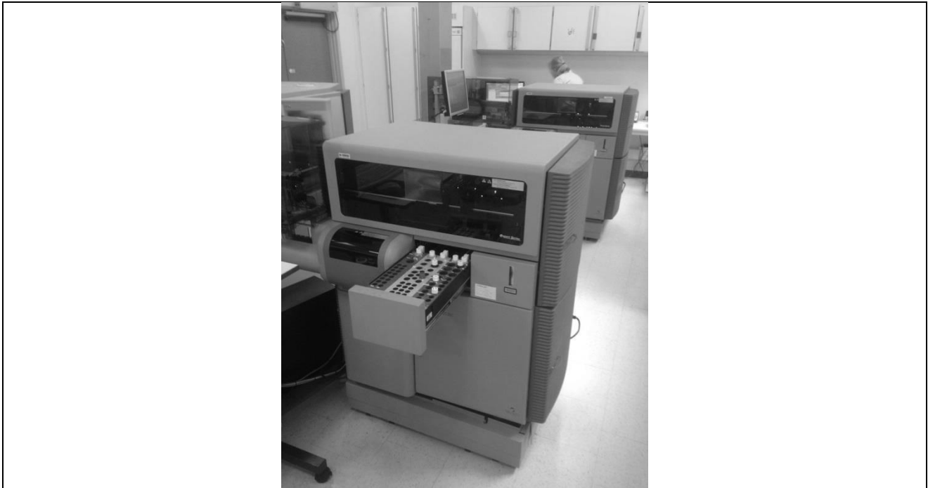
Figure 2. The STA-R unit. The tray is open as reactor fluids are being replenished.
