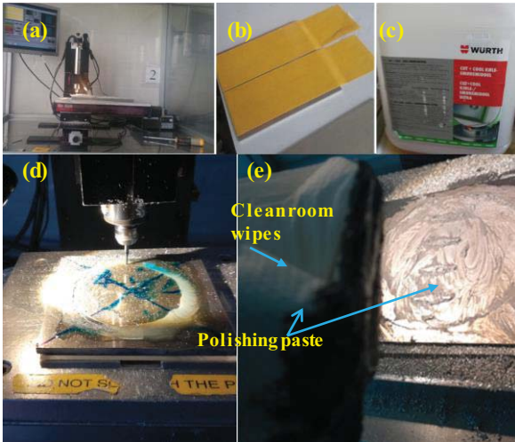
Figure 3: Digital pictures of (a) Milling machine. (b) Attached double-sided tapes on the backside of the Al-plate to immobilize it on the milling stage. (c) Cooling oil from Wurth, Germany. (d) Milling stage where the Al-plate is attached and the cooling oil is applied on the Al-plate surface. (e) Applying the polishing paste after bulk milling using Autosol ALUMINUM polishing paste and cleanroom paper.
