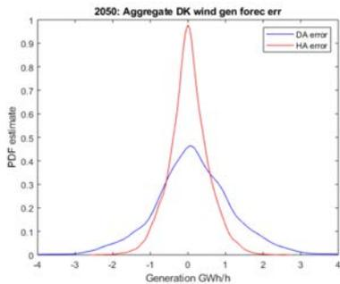
Figure 1. Day-ahead and Hour-ahead wind forecasts error [1]
