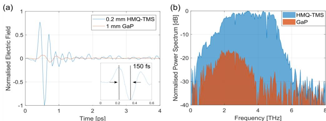
Figure 1. THz waveforms in the time domain (a) and their corresponding spectra (b).
