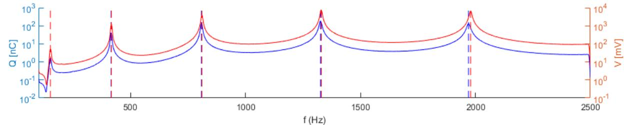
**Figure 2.** FRF for electric current and voltage for the left piezoceramic patch pair on the free beam Fig. 1(b).
