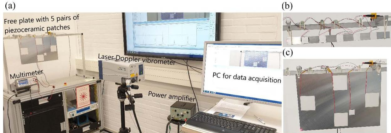
**Figure 1.** Experimental setup (a) and close-up of the tested free (b) beam and (c) plate with five pairs of co-located piezoceramic patches.
