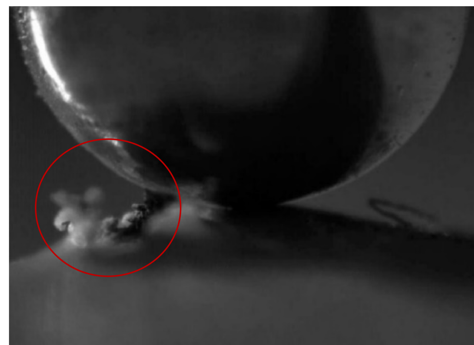
Fig. 4. Film sample after breakdown, with a hole (marked with red circle). Electrode diameter: 2mm.
